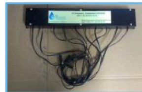
Charging Station Multi-household energy supply electronics
